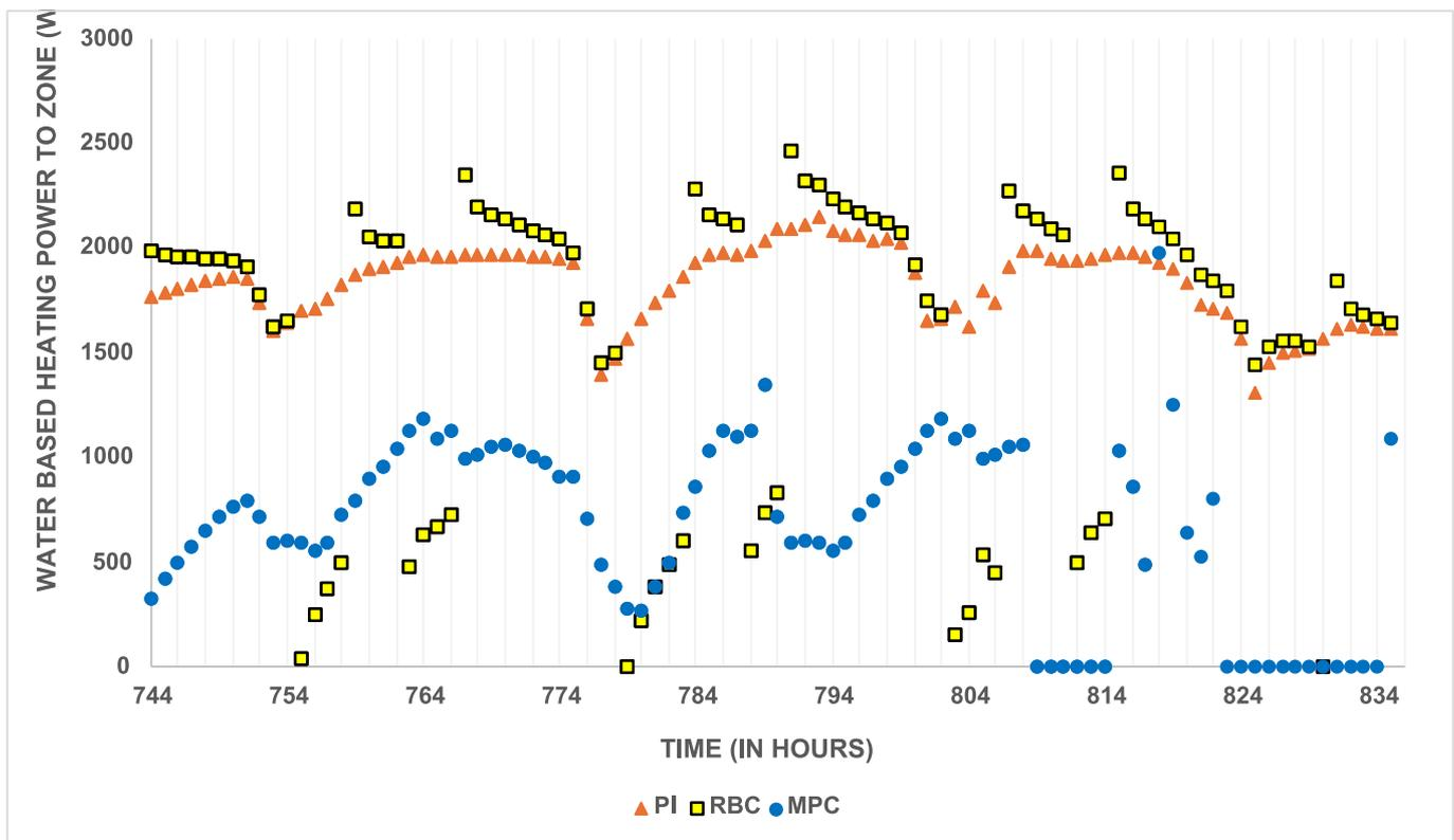
Fig. 8. Operational behaviour of the heating system in building B1 versus time for the three control strategies.
