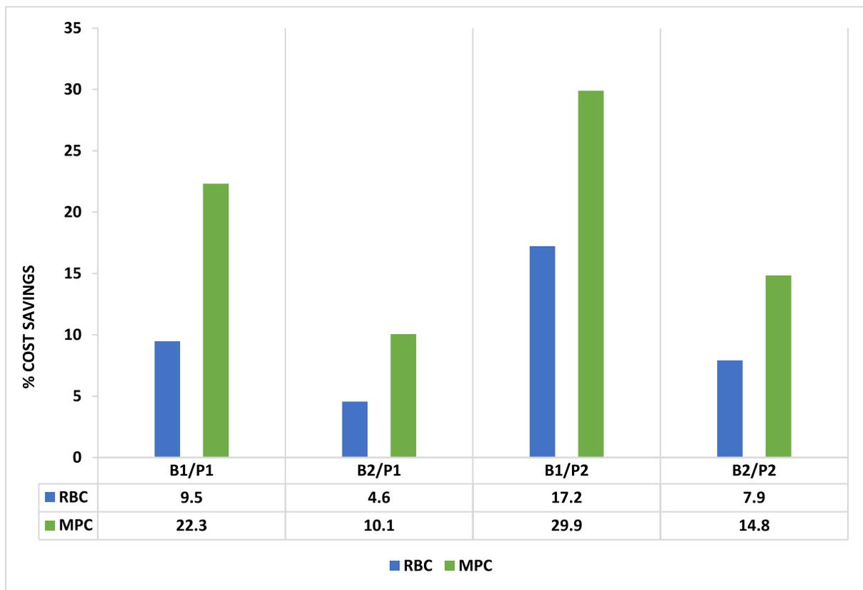
Fig. 11. Total Cost savings in % (as compared to PI control) when the RBC and MPC are implemented for the two buildings (B1, B2) for the two electricity price levels (P1, P2).
