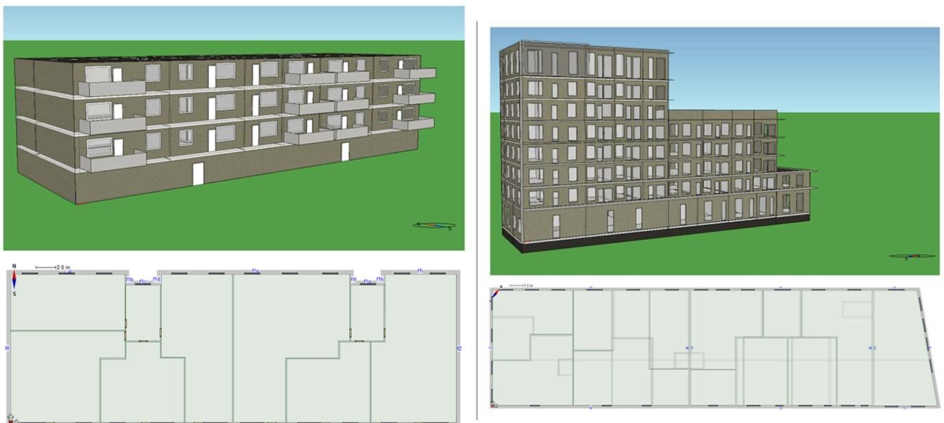
**Fig. 1.** The 1970s-era, poorly insulated building B1 (left) and the modern PEB B2 (right) in Helsinki modelled using IDA ICE.
