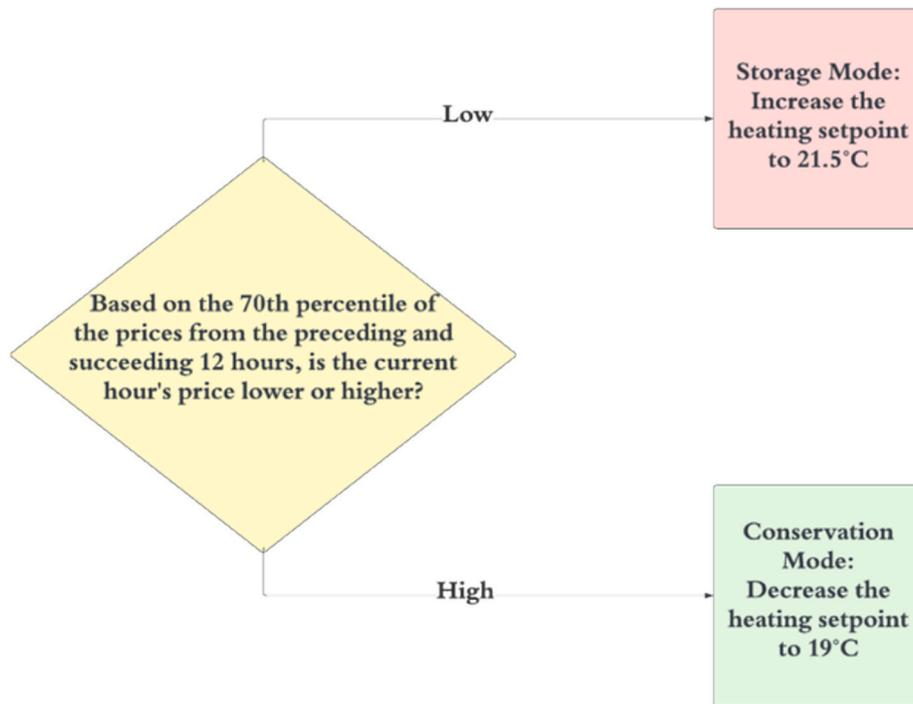
Fig. 6. The workflow for the RBC strategy utilised in this work.
