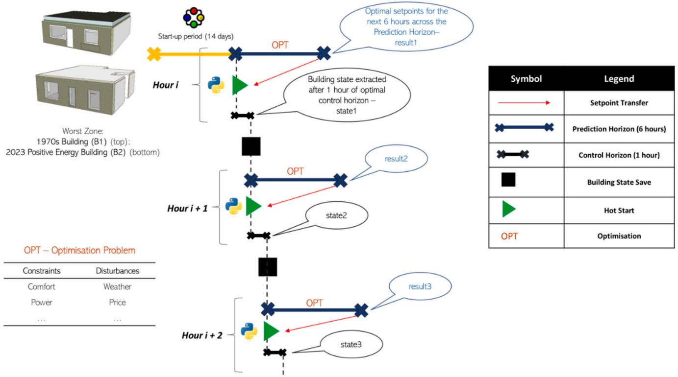
Fig. 7. The workflow for implementing the MPC used in this work, in co-simulation with IDA ICE.
